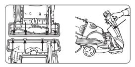
Replace all three (3) screws to secure nozzle guard.
